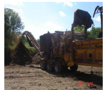
Resident generated yard waste tub ground into mulch product
